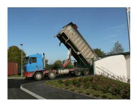
It must be borne in mind that there are numerous types and sizes of tractor and trailer and therefore combinations of the two. Because the trailer or lorry is not dedicated to the delivery of wood chip this is often the least expensive form of delivery and due to the availability of the equipment a customer generally has a wide choice of suppliers.
