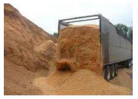
A principal advantage is that the high speed of unloading means that disruption and noise on site is relatively minor. Travelling distances need to be kept to a minimum, ideally not much more than 20-30 miles, mainly because the low bulk density limits the carrying capacity and pushes up the cost per tonne.
